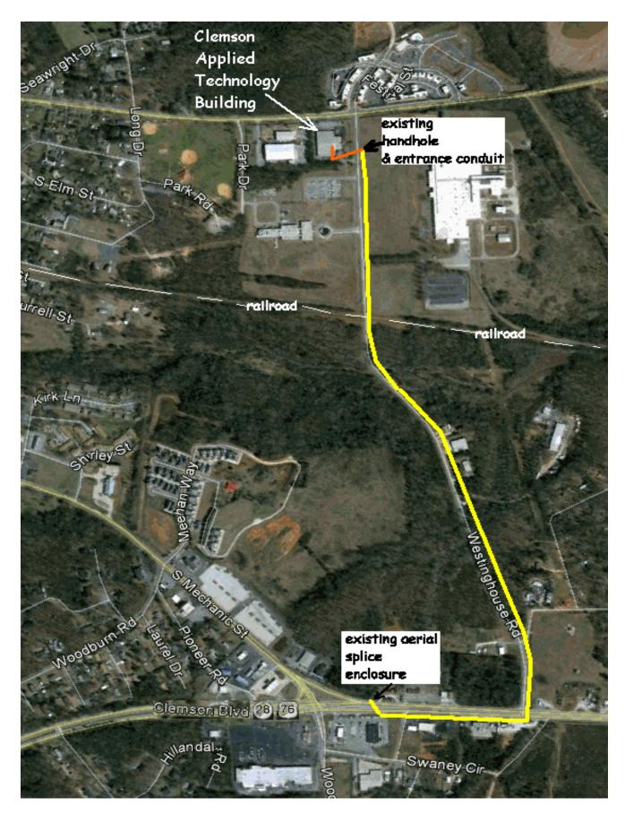
Enter the existing Clemson enclosure along Highway 76 near the intersection of S. Mechanics St. and splice 4 strands of the 48 strand fiber onto the Clemson owned 96 strand fiber. Terminate the other end inside the CAT building in designated location on LC UniCam connectors. Secure inside enclosure per manufacturers recommended procedures and industry standards.
