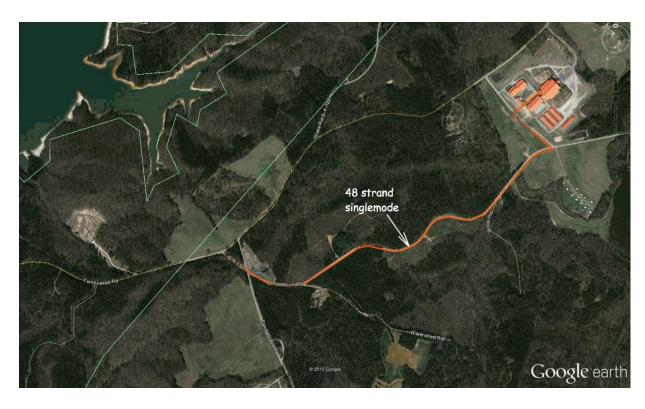
End the 48 strand fiber as shown near the intersection of Twins Lakes Rd. Splice on 24 strand singlemode and continue aerial approximately 3500 feet south along Twin Lakes Rd to the Fire Tower Service Rd as shown.
